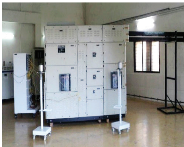
Panel temperature rise test
