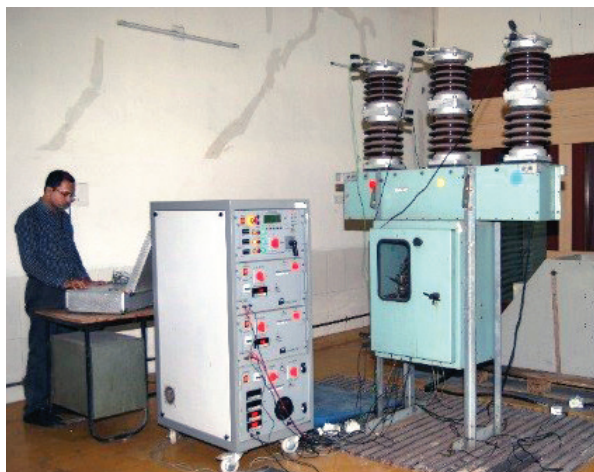
HT breaker mechanical endurance test setup
